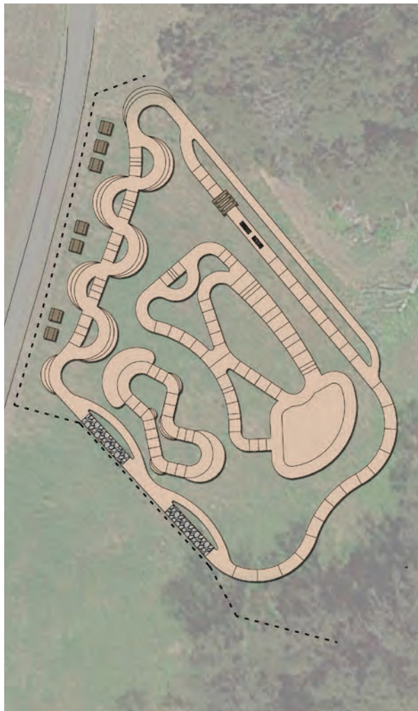
Figure 5-2: Pump Track Layout
