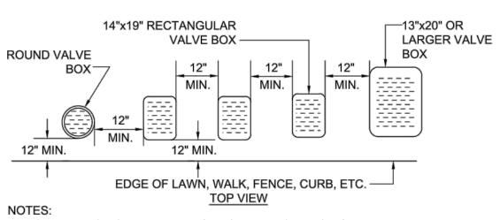
1. CENTER BOX OVER VALVE TO FACILITATE SERVICING VALVE. 2. SET BOXES 1" ABOVE FINISH GRADE OR MULCH COVER IN GROUND COVER/SHRUB AREA AND FLUSH WITH FINISH GRADE IN TURF AREA.
