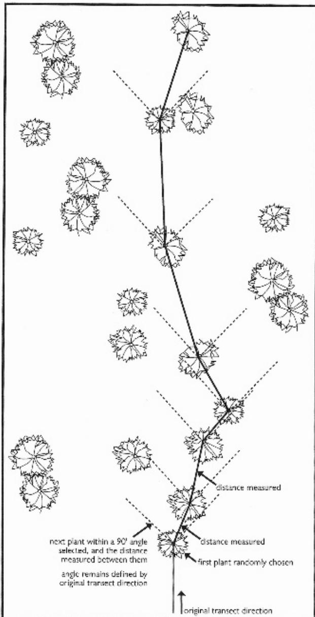
Figure 3-8: Plotless Wandering Quarter Distance Method, excerpted from Elzinga et al. 1998.
