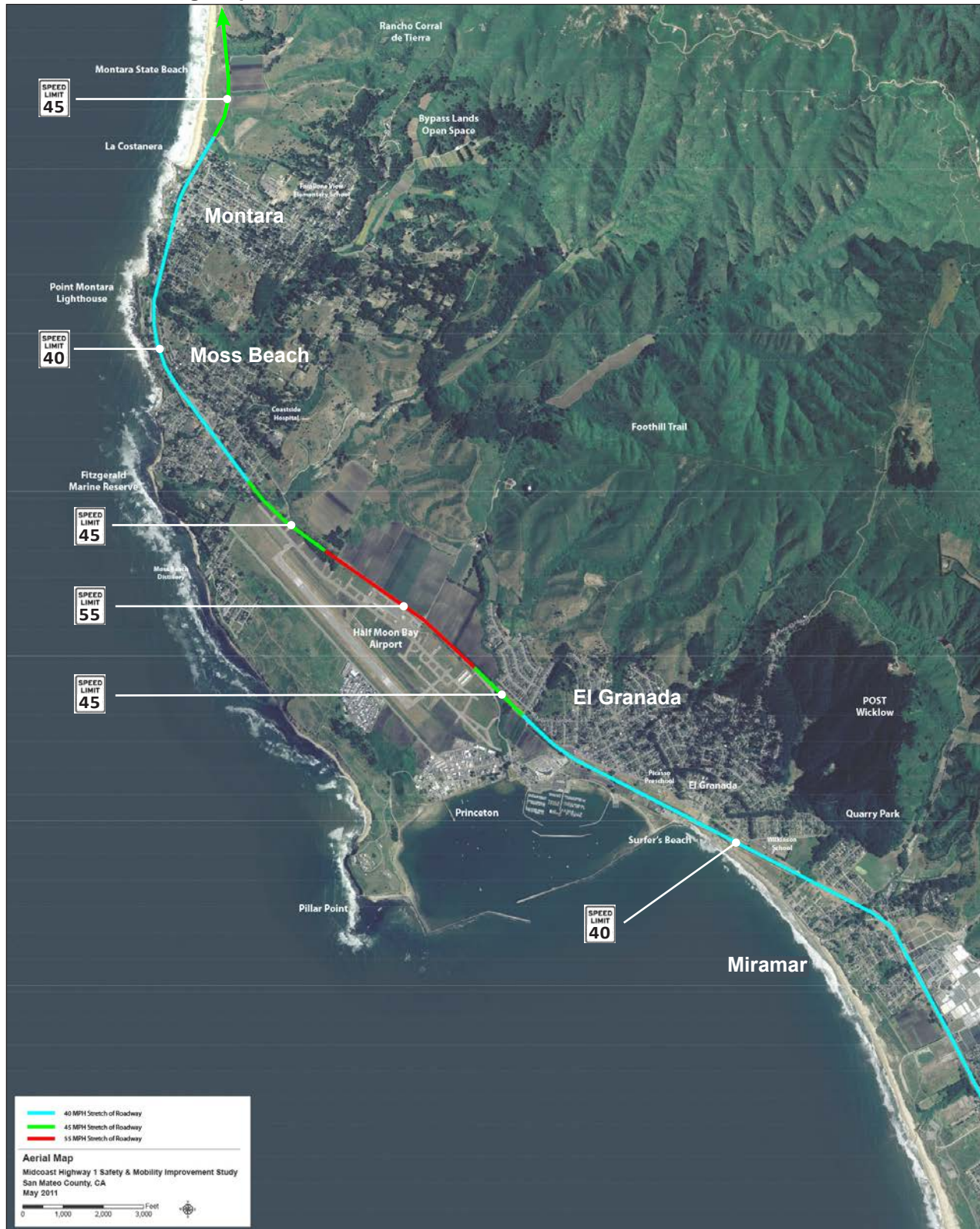
The image above shows suggested targets for motor speeds through Community and Fringe zones for increased safety and flexibility in highway design and operations.
